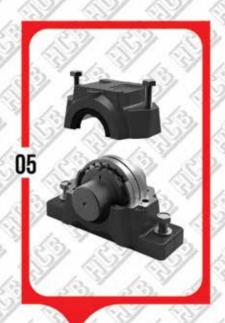
place the cap on the base tighten cap bolts and attachment bolts
