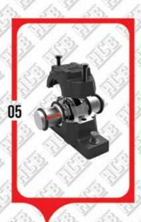
place the cap on to the base tighten cap bolts and attachment bolts do not forget to grease washer's contact surface for the V-ring
